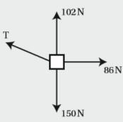
Find the magnitude of the force marked **T** and the angle it makes with the 102 N force.
