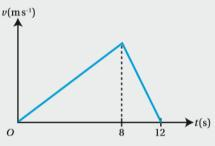
Find the acceleration of the particle during the final 4 seconds.
